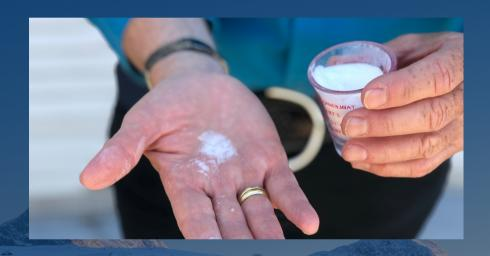
We are proposing the deployment of a thin layer of very small hollow glass microspheres across targeted regions of the Arctic, improving the reflectivity of sea ice. This approach mimics natural processes that reflect solar energy out of our atmosphere.
